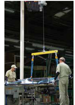
Invert large window glass by using only one sling belt
