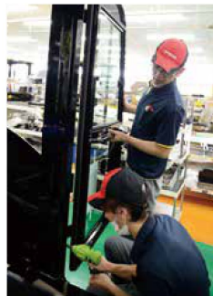
Bolt tightening work that used to be done by two persons can now be done by one
